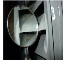
Figure 7 - Blade Tip Trailing Edge Erosion
