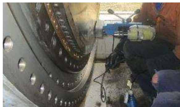
Figure 4: A magnet base drill used on a rotor disc
