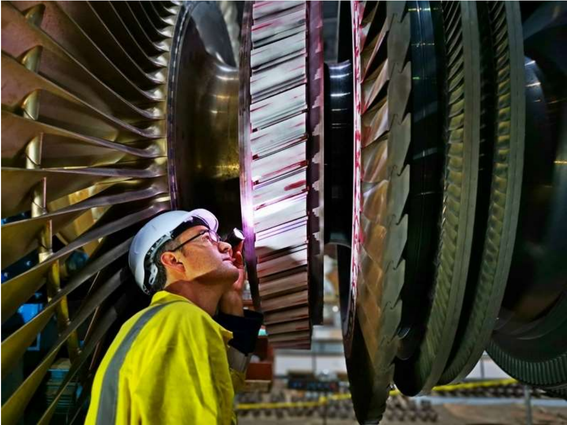
Row L-1 blade root inspection – Prior to reblading
