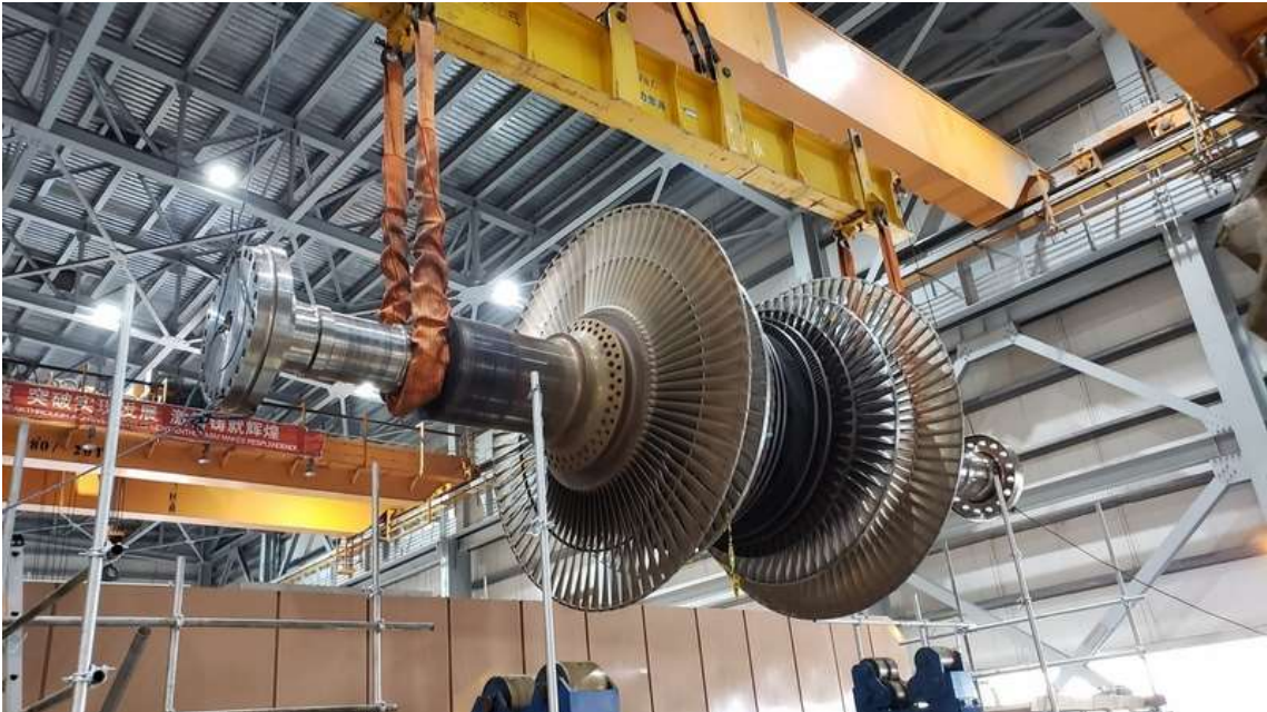
Turbine LP rotor repositioning after reblading.
