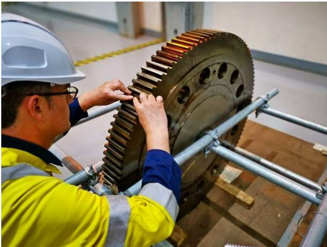
Turning Gear bull gear inspection
