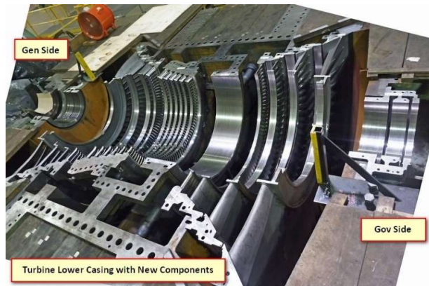
Picture of the turbine lower casing with new components installed
