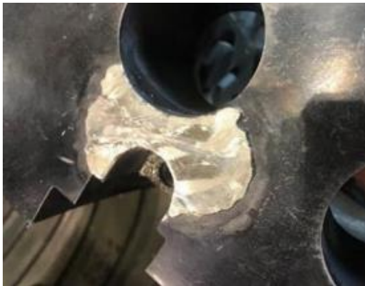
Figure 5 The leak area build up with Brazing
