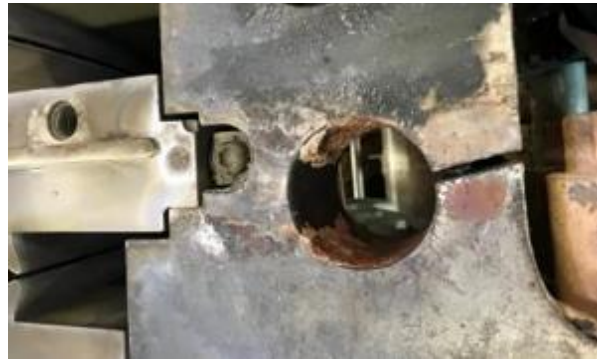
Figure 2 Leak position in the bottom casing
