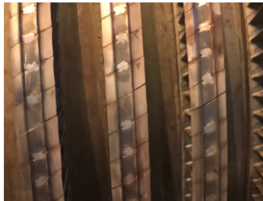
Figure 7 Rotor shrouding worked down
